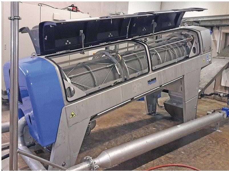
Figure 13 Proposed Screw Press in the new Centrifuge building.
